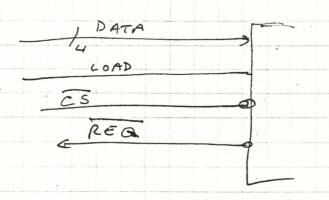
LOAD CAUSES DATA TO BE TRASFERRED
